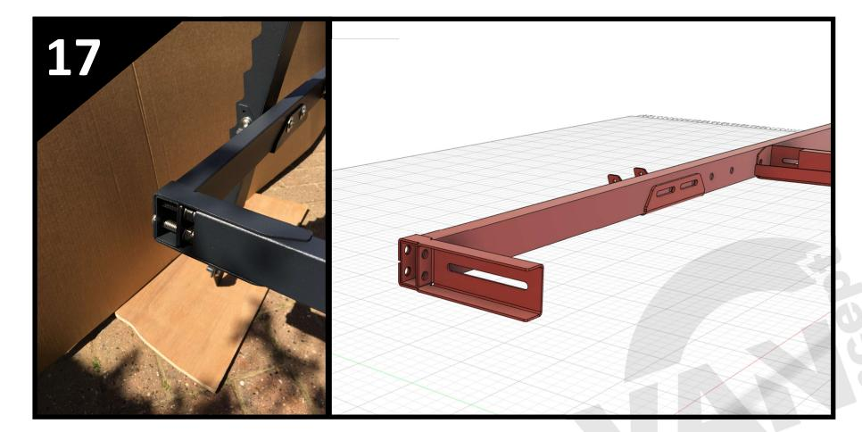
At the front, position both the Bed Frame Bracket Front brackets over the ends of the Side Beams (note orientation), before fitting 1x M8 x 40mm button head bolt, with 2x M8 washers and 1x M8 nyloc nut through each hole, on both brackets as shown, before tightening.
